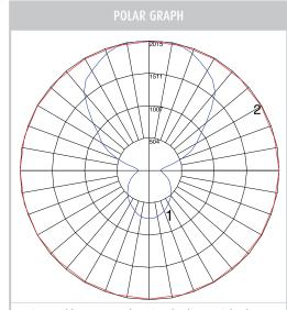
Maximum Candela = 2014.5 Located At Horizontal Angle = 0, Vertical Angle = 175 #1 - Vertical Plane Through Horizontal Angles (0 - 180) (Through Max. Cd.) #2 - Horizontal Cone Through Vertical Angle (175) (Through Max. Cd.)
